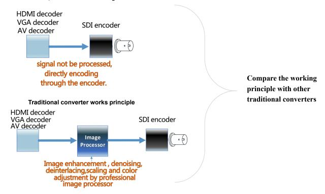
SD/HD/3G SDI - HDMI&VGA&CVBS converter working principle
