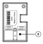
2 Power input port ⑤ Indicator of power input ③ IR/TX **6** CAT5e/6
